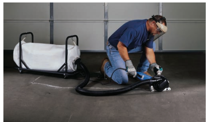
Hand-held crack chasing saw shown with bag wagon.
